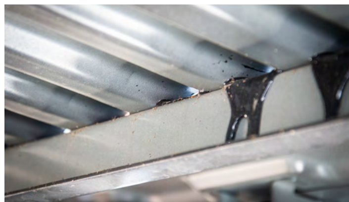
Below: An example of a hidden air "leak" where the load-bin meets the cab on an LC79. Often, it may look like the rubberising has sealed the gaps from the top, but a view from the undercarriage reveals a different picture.
