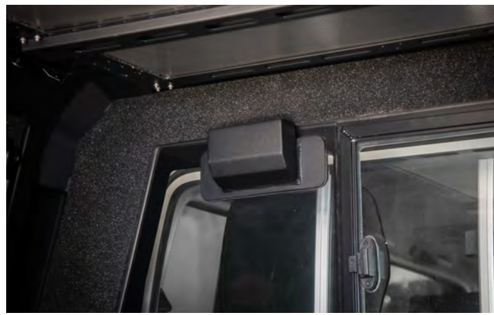
Above & Below: The pressure vent only works if the air volume entering the canopy is greater than the volume exiting through holes and gaps, which aren't always obvious. Every opening should be sealed.
