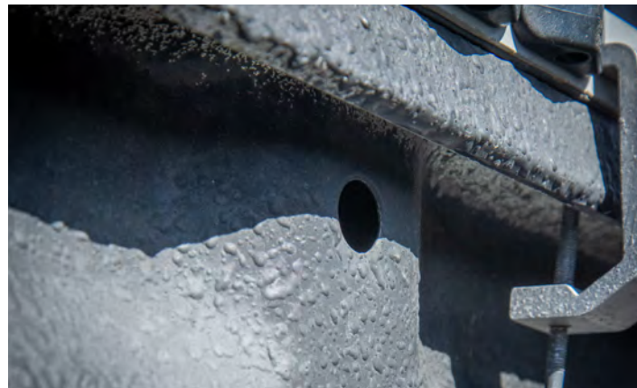
Below: An example of a hidden air "leak" where the load-bin meets the cab on an LC79. Often, it may look like the rubberising has sealed the gaps from the top, but a view from the undercarriage reveals a different picture.
