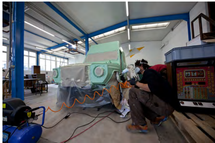
Above: Applying the new paint coat with the spray gun.
